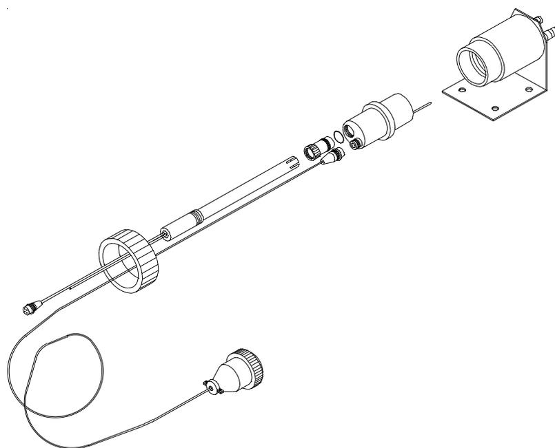
Figure 3.2 - pH Adapter Plug Assembly
