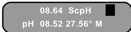
The Black Square indicates that the Mark 22 is in the data LOG mode of operation. Pressing the FREE key will display the amount of memory remaining for data storage in terms of logging hours remaining and then return to Log Mode. The LOG mode may be paused by depressing the PAUSE key. Logging will be suspended until the RESUME key is depressed. The upper right corner of the display will show a letter " p " instead of the black square when the Mark 22 is in the paused state of the Log Mode.
