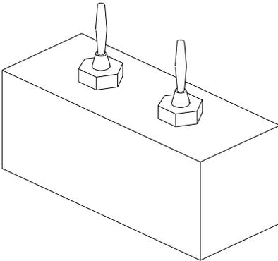
**Calibration Plugs for ZERO (P/N 400550) and SPAN (P/N 400549)**
