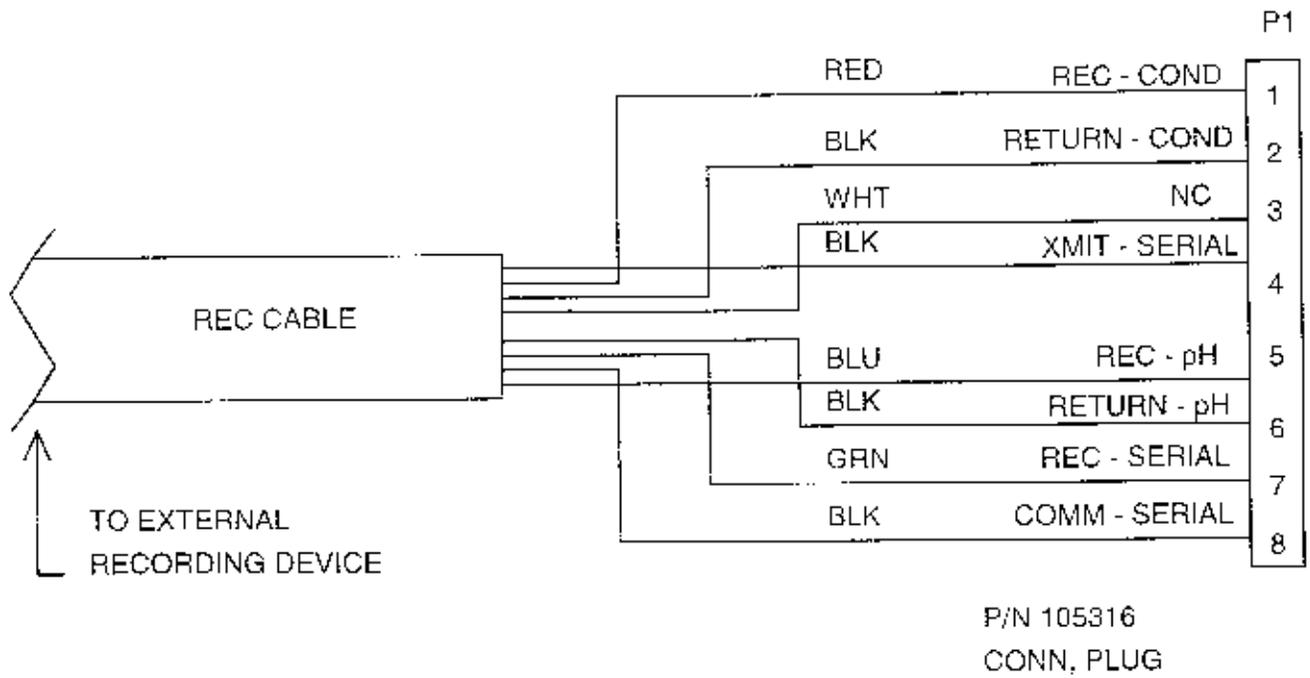
**Figure 4.3 - Analog Recorder Output Hook-Up**
