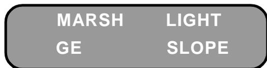
The operator must use the UP and DOWN ARROW Keys, to navigate the display and highlight the desired compensation formula. The option is chosen by user when the SEECT Key is depressed while one of the formulas is highlighted.
