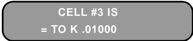
and the "1" will be flashing. You can now alter the value of the flashing digit by pressing the UP or DOWN ARROW key. You can then move forward to the next digit by pressing the SELECT key and move back to a previous digit by pressing the EXIT key.
