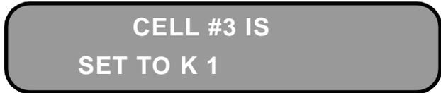
with the "K 1" prompt flashing. Using the UP and DOWN ARROW keys, change the flashing "K" factor until it reads "K .01". Now press the SELECT key. The display will now indicate:
